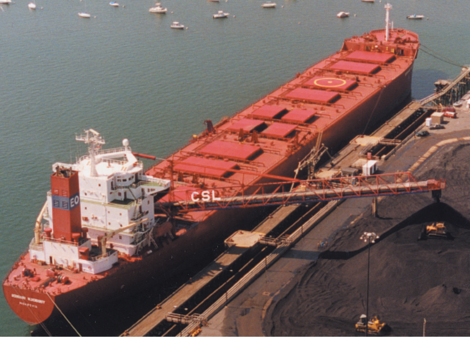
The Bernhard Oldendorff discharges onto an open stockpile at a power plant at Salem, MA.
