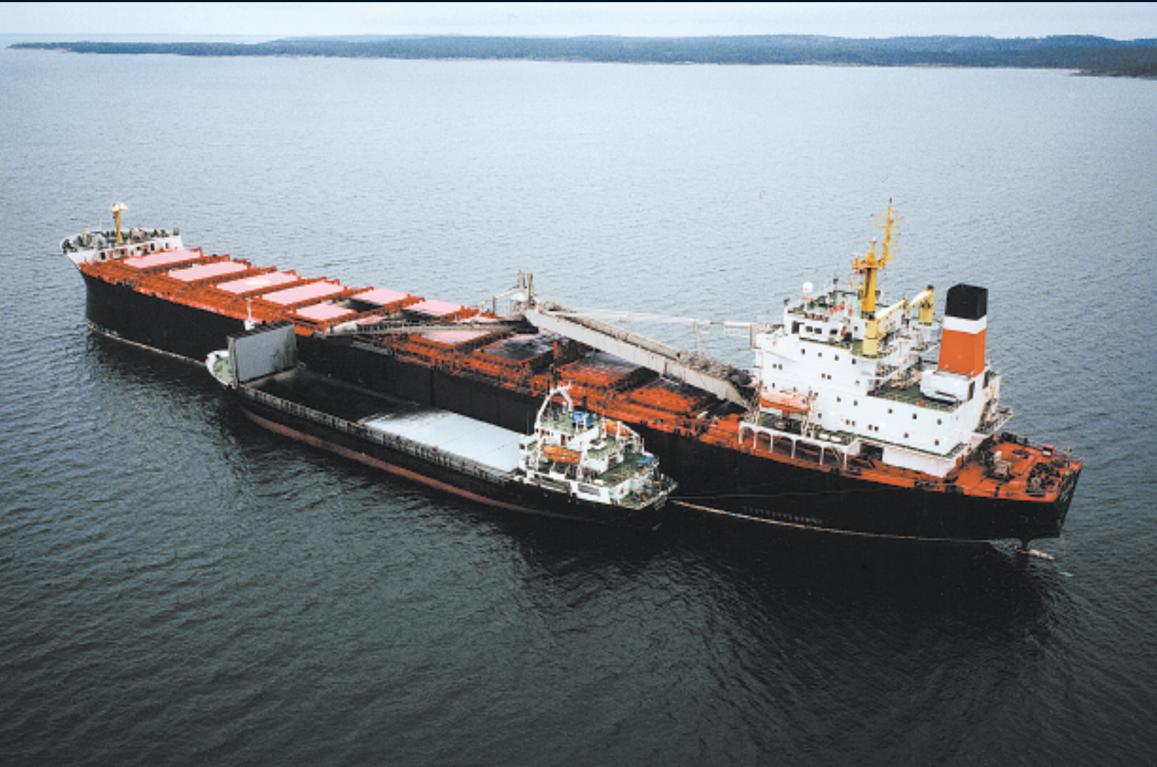
The CSL Atlas uses her articulated boom to unload into a gearless bulker alongside.
