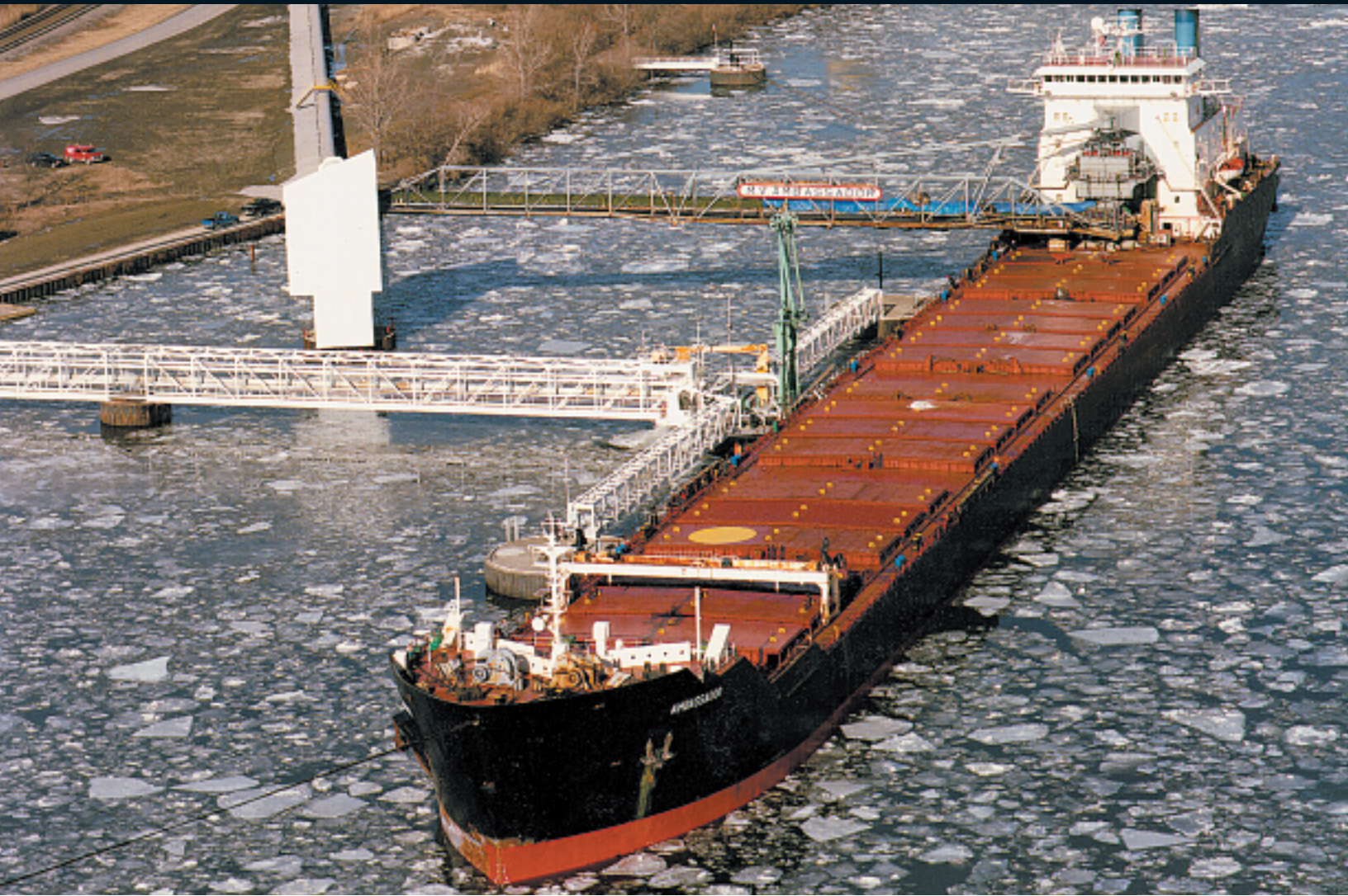
Discharging into an enclosed hopper, at a power station on the Hudson River.
